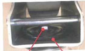
Castor mounting bolt Swivel bearing head should feel free to rotate and not loose
