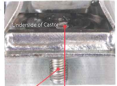
Castor mounting bolt Swivel bearing head should feel free to rotate and not loose
