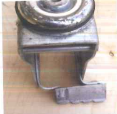
Foot pedal distortion as a result of a significant frontal impact; it is likely the top plate and bearing will be distorted as well.
